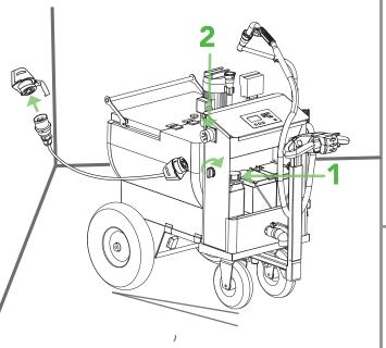
SET Cleaning Once before commissioning & after each feeding Attention! First insert the cleaning nozzle loosely into the opening provided, then attach dosing arm to it. Enter
