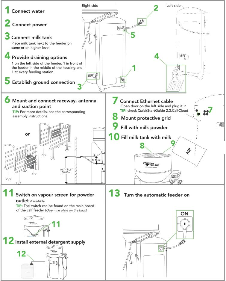
This checklist refers to the basic equipment of the calf feeder. Not all available functions of the automatic feeder or the extensions can be shown. For detailed information and valid warnings as well as safety instructions, please refer to the instructions manual. (Status 21/07)
