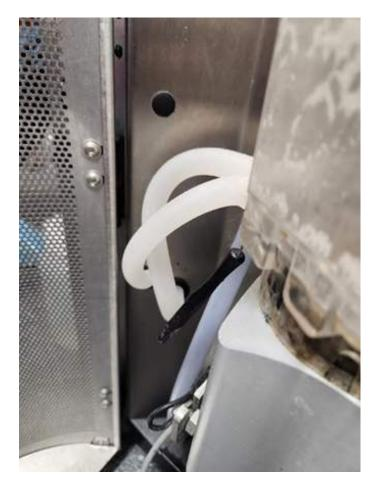
See the hoses coming off the mixer jar and that little rubber band? The hoses should be threaded through this rubber band when they are changed. Why? If the hoses touch the screen door when it's closed, this interferes with accurate measurement of delivered powder and detracts from mixing accuracy. Little things can add up, particularly in the summer. Paying attention to details keeps the feeder operating at peak efficiency and effectiveness.
