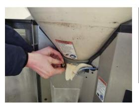
Another management task which should be repeated at least monthly is to clean the orifice where the powder is delivered. Unscrew the black knob and remove this metal insert. Hand clean it and reinstall it. This seemingly small task improves accuracy and precision of powder delivery.
