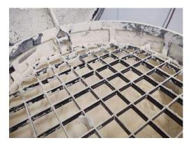
Although milk replacer powder has extremely low levels of bacteria it's a good idea to occasionally clean the "hopper" where the powder is stored prior to delivery to the calf. Moisture is always present near the feeder and milk replacer powder is very hygroscopic meaning it absorbs water. Wait until the hopper is nearly empty and then remove powder residue and wipe the surface with a damp cloth. Allow to dry before adding more powder. This will be more important to do during warm weather!
