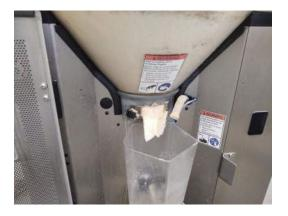
Once again, the failure to perform some simple maintenance can make all the difference. Use the plastic wand attached just to the left of the mixer bowl to remove this "bear" as it can impair accuracy of powder deliver.
